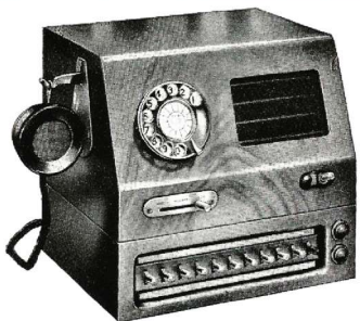
Fig. 11. Loud-Speaking Cabinet with Key-Calling facilities.
